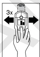
To localise the object precisely, press the "**ZOOM**" button **4** and keep it pressed while repeatedly (3x) moving the measuring tool over the object. The "Zoom" function indicator **d** appears in the display. The "Zoom" measuring indicator **e** has the greatest amplitude over the centre of the metal object.
